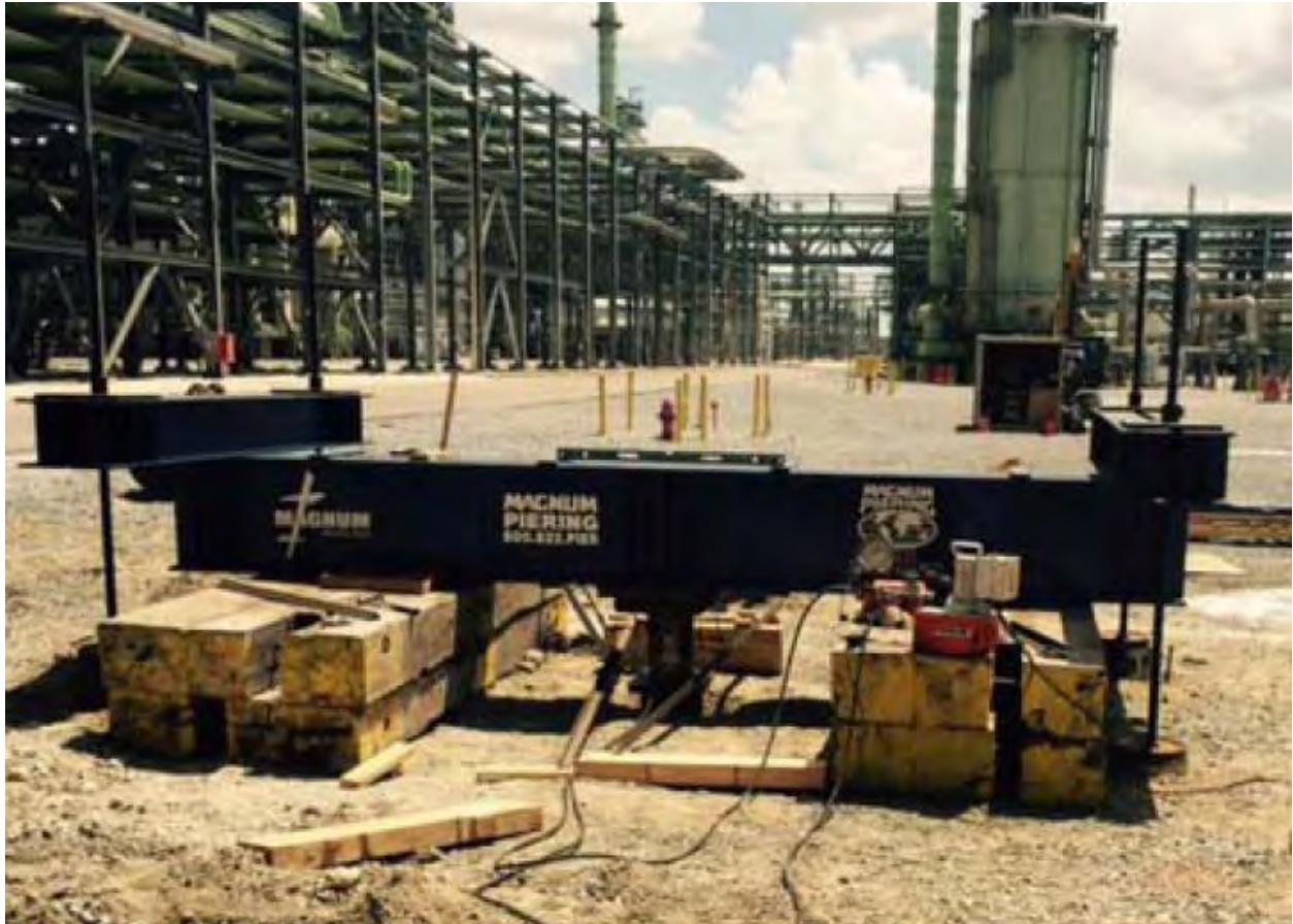
Fig. 7. Compression Load Test (Courtesy of Magnum Piering, Inc.)
